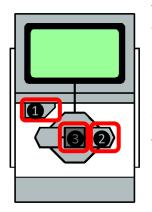
To **turn** the **EV3 Brick** off, press the Back button until you see the Shut Down screen.
